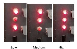
5. Press and hold button 4 to increase temperature (flame height will increase), press and hold button 5 to decrease temperature (flame height will decrease)
